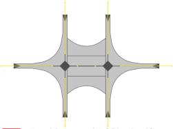
Expand the ropes to their full length and fix them to the ground according to the above drawing.
