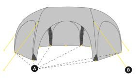
At the end, stabilize the tent. Attach the legs to the ground using straight pegs.
