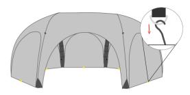
The zipped walls should be attached to the ground with straight pegs.
