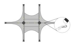
Spread out flat and clip the ropes to the eyelets using carabiners.
